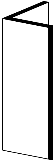
ANGLE SECTION 60 x 60 x 6 mm
