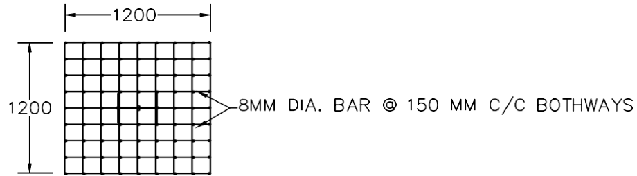
DETAILS OF HORIZONTAL & VERTICAL BARS ANCHORING BEAM
