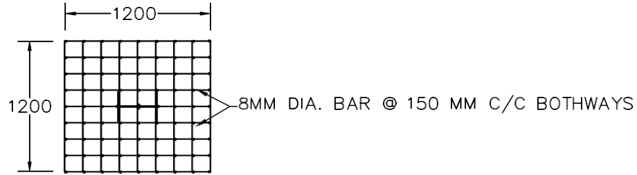
DETAILS OF HORIZONTAL & VERTICAL BARS ANCHORING BEAM
